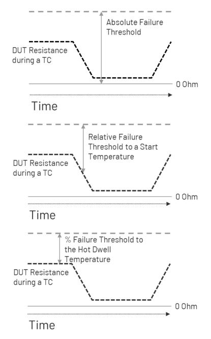
Figure 1: The top image shows an absolute resistance value for a failure definition. The middle image has the baseline reference resistance, for example, at room temperature while the entire resistance swing from Hot to Cold will be higher and lower than the baseline. The bottom image shows a reference resistance set at the Hot temperature.
