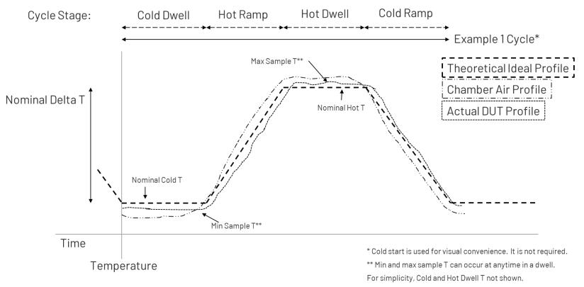
Figure 3: A temperature cycle and its terms are shown for reference.
