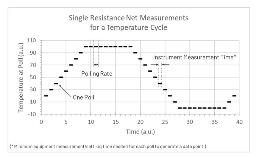
Figure 2: An example of polls, resistance measurements, during a temperature cycle for a single device or a single subnet.
